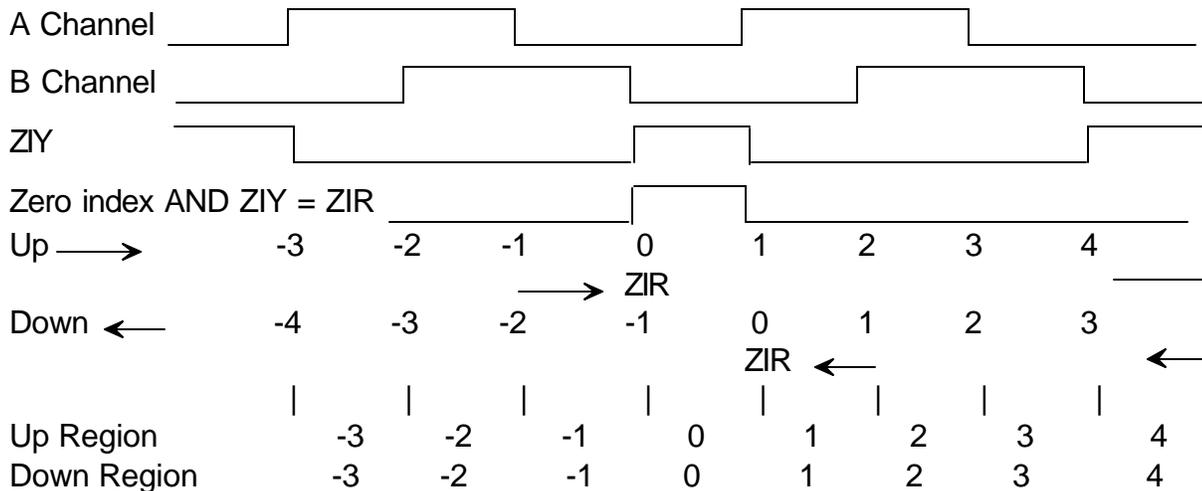
By ANDing the zero index signal with the A & B channels, there is no regional discrepancy
