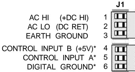
\*Note: Non-isolated external control inputs A and B are menu selectable.
