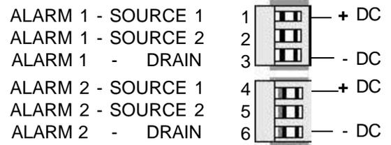
\* This configuration is directly compatible with the optotransistor output board.
