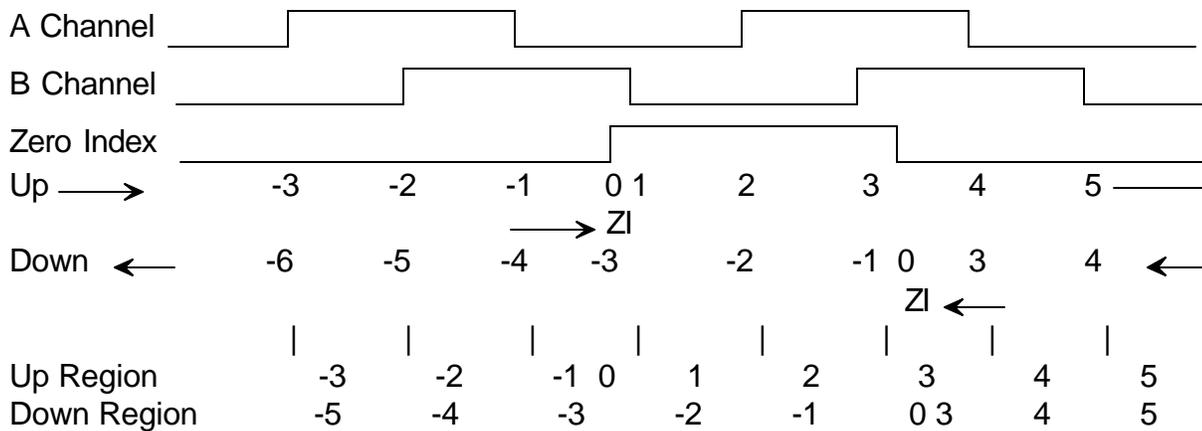
It follows that a wide zero index signal causes a discrepancy in the count in the regions between transitions when counting up and counting down. To correct this situation, AND the zero index signal with the A & B channel signals. Assume for this example the zero index is ANDed with the inverse of A ( $\bar{A}$ ) and the inverse of B ( $\bar{B}$ ) to produce ZIY as shown below.
